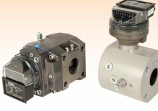
Installation of FMG rotary meters can be horizontal or vertical. Since the meter is designed for multi position, consideration need only be given to the arrows showing the flow direction. After the meter is installed, the index can be rotated to the correct position. The index can be rotated over 350°. FMG rotary meters can be metrological sealed to suit various conditions from total flexibility to highly tamper proof.
