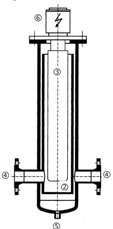
heating insert is surrounded directly by natural gas. The maximum surface temperature is chosen so that the temperature can not be higher than the allowed one - according to the ex-protection - also when there is no gas flow. The apparatus will be designed according to the clients requirements. An inline design, as a standard feature in many reducing stations, can be delivered as well as any other positions of nozzles.
