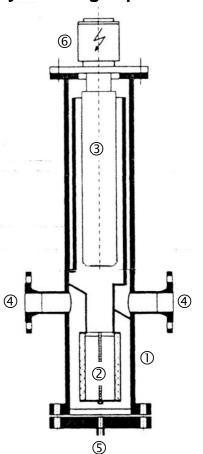
An especially effective and proven solution is the com-bination of heat exchanger type WAT- EX and cartridge filter. So the filtering of the gas as well as the heating can be executed in one apparatus.
